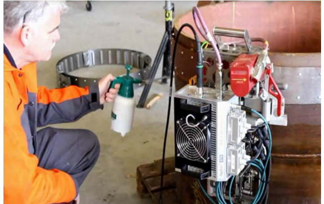
IWEX 3D Imager mounted on the AUT RTD RotoScan system
