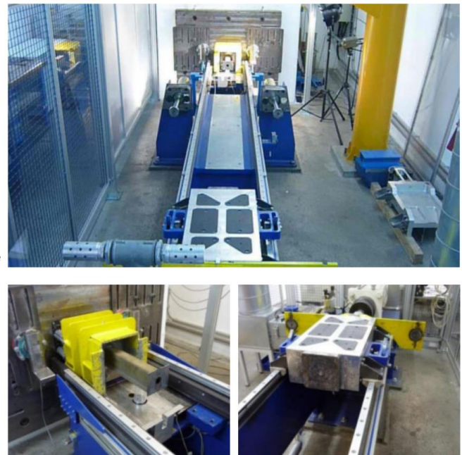
Fig. 4 Axial impact test set-up on a DP1000 steel beam used as a validation method.
