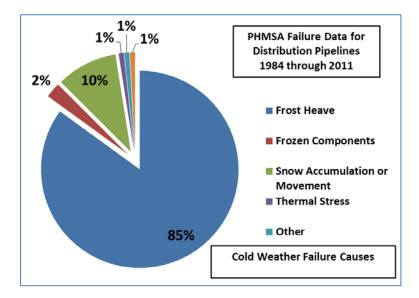
Figure 2. PHMSA Cold Weather Failure Causes
