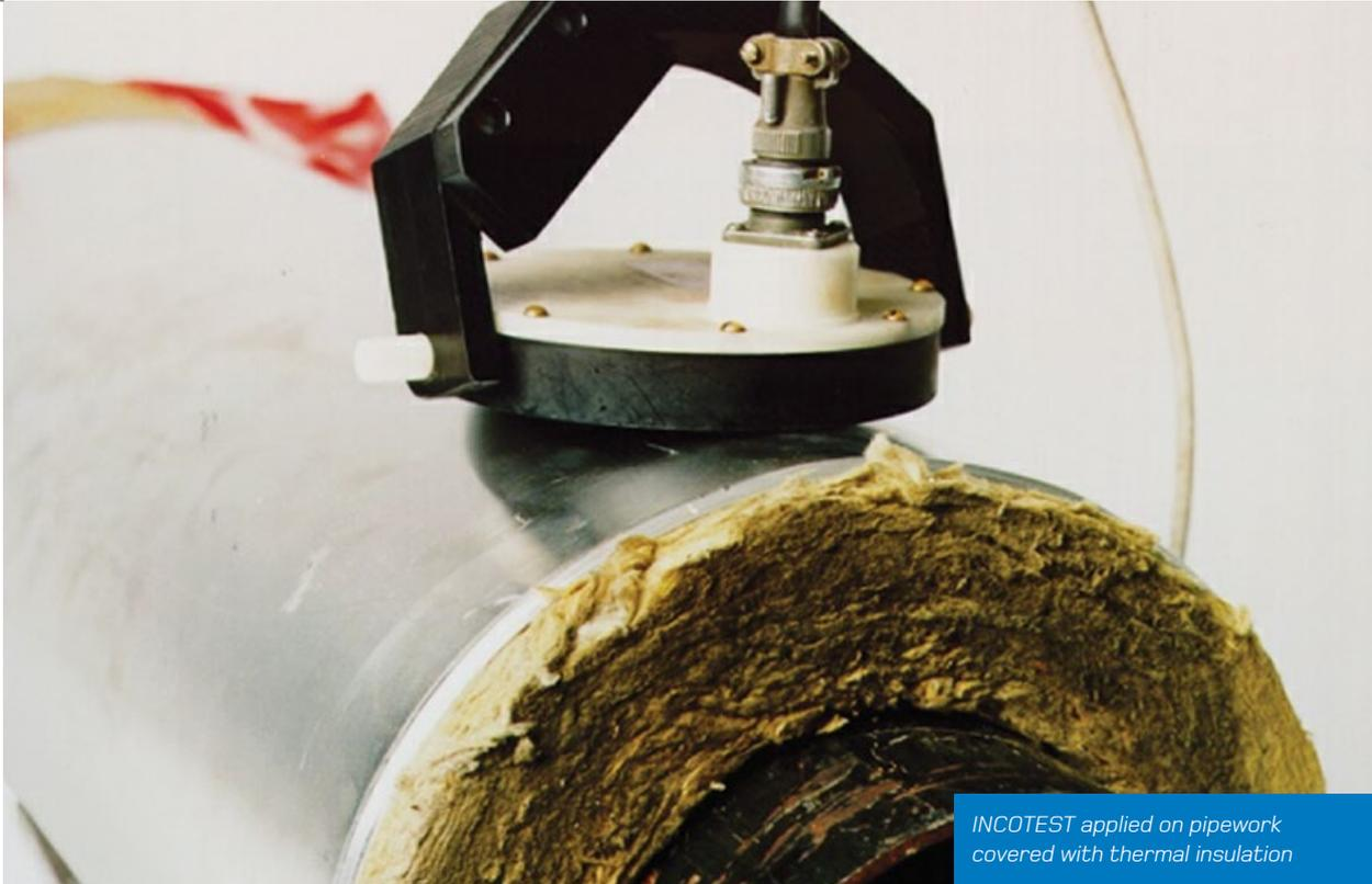
*INCOTEST applied on pipework covered with thermal insulation*
