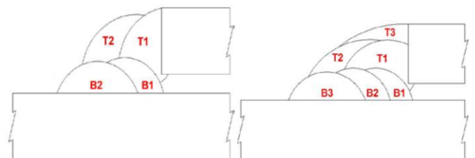
Figure 2. Fillet Weld Deposition Sequence
