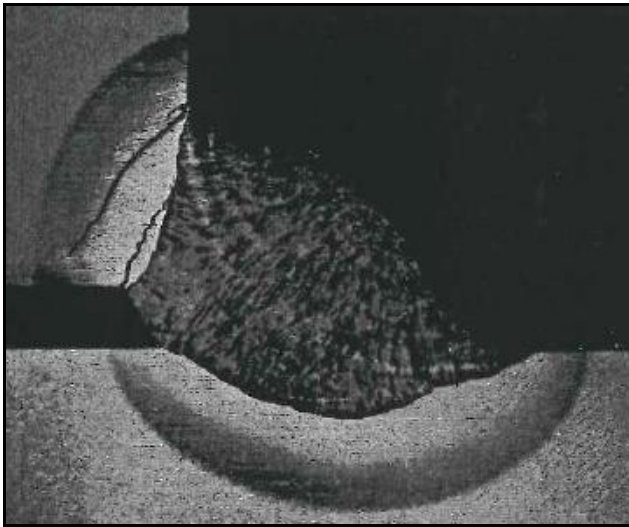
Figure 6. Image of Sleeve HAZ Hydrogen Cracks [7]
