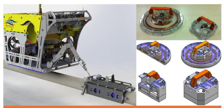
A pioneering tool for the ROV deepwater inspection of non-piggable pipelines, called RTD INCOTEST, is proving to be a more cost-effective, faster and a safer way to detect corrosion. Through a new partnership between Applus RTD and Delta SubSea, this new one-of-a-kind deepwater tool is being introduced in the marketplace. The Applus RTD INCOTEST tool uses Pulsed Eddy Current testing to detect surface and subsurface corrosion in thin and thick-walled pipelines and vessels.
