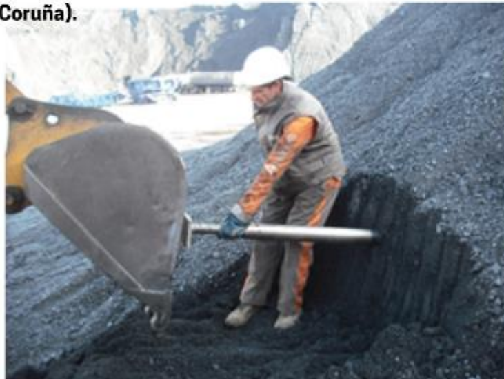
COAL SAMPLING IN THERMOELECTRIC PLANT IN CARBONERAS (Almería)
