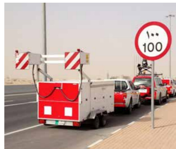
Laser Crack Measurement System and LIDAR system in a highway, Qatar
