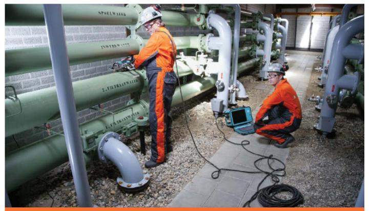
Eddy current testing is used to detect discontinuities in assets such as pipes and tubing by subjecting them to a strong external magnetic field.
