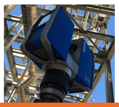
The FARO Laser Scanner Focus is an advanced 3D surveying system that captures three dimensional measurements, quickly and accurately.
